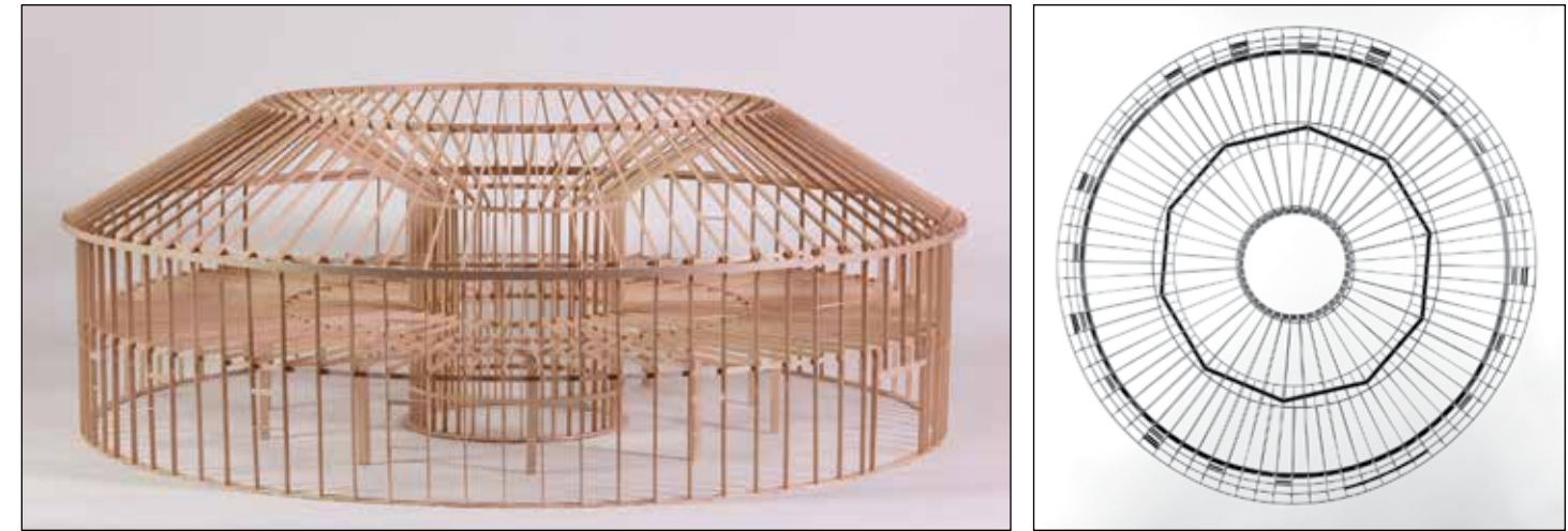
Figures I.11 and I.12: Model (left) and aerial perspective of the intricate, radial wood framing of the Jim Kaney Round Barn, Aledine, Illinois, built in 1905. The Kaney Barn design is unique, as the inner circular segment—usually a silo supporting a dome roof—is actually concave and funnels rainwater for the animals. This model was on display at the Architecture and Design Museum in Palm Springs, California in spring 2023, and was featured as one of ten models in an international exhibition on the importance of wood framing in the development of the United States. Images courtesy of American Framing.
