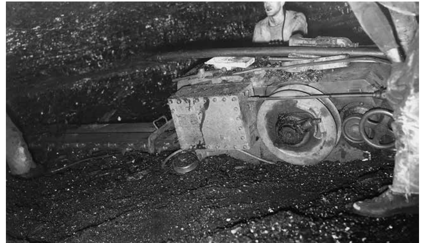
Miners operate a shortwall mining machine in Ronald's No. 3 mine. The use of coal cutting machinery did not come to the Roslyn-Cle Elum coal field until the late 1920s since the machines were designed for use in relatively flat areas. The slope of many of the state's coal fields presented difficult engineering challenges. Courtesy of Roslyn Public Library, Roslyn Heritage Collection, by permission of Frank Schuchman
